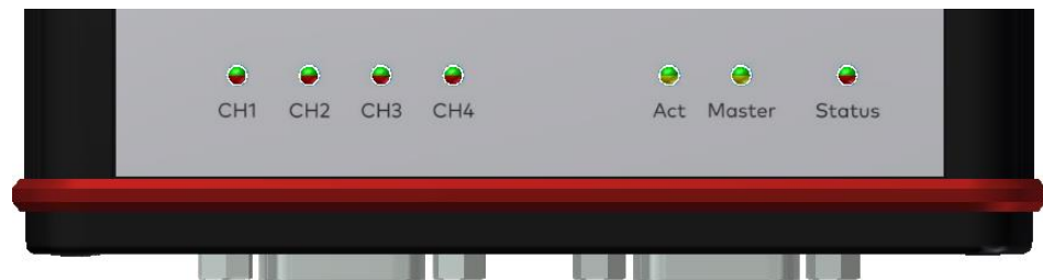
Figure 11: Top LEDs on VN7640
