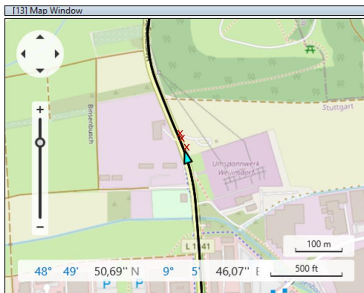
Figure 23: The total distance with the current position of the vehicle is displayed. The red crosses represent detected vehicles.
