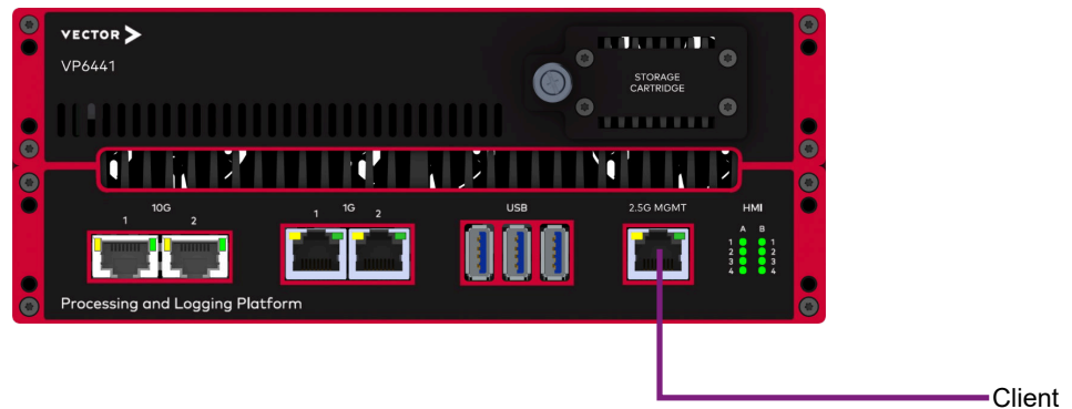
Figure 38: MGMT port connected to client
