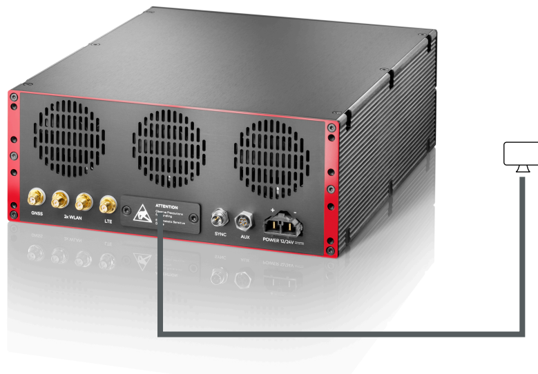
Figure 37: Connecting monitor (Mini-DP connector behind cover)
