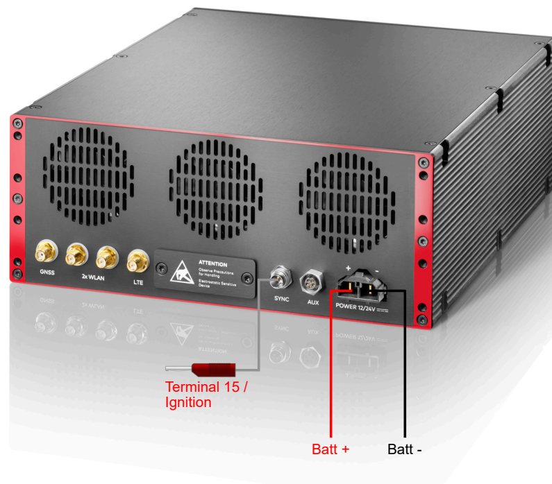
Figure 30: Connecting VP6400 to power supply
