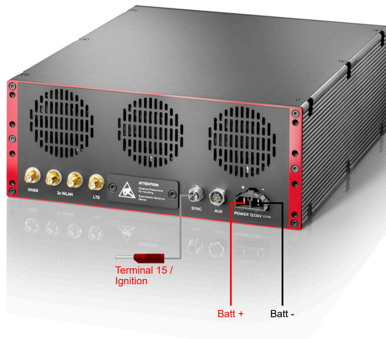
Figure 35: Connecting VP6400 to power supply
