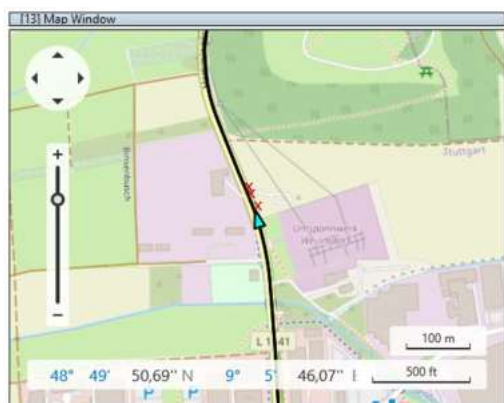
Bild 11: The total route with the current position of the vehicle is displayed. With the "Driver Assistance" option, detected vehicles can be visualized as red crosses, for example, as shown here.
