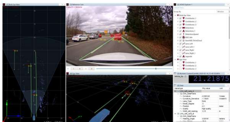
Bild 13: Option "Driver Assistance" - Object verification for driver assistance systems and optimization of image processing algorithms
