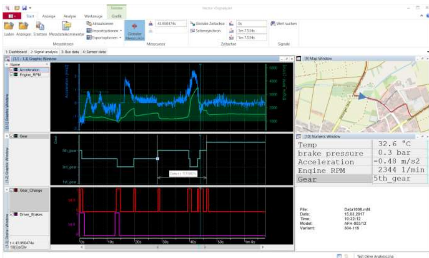
Bild 1: Convenient display and evaluation of measurement data with vSignalizer
