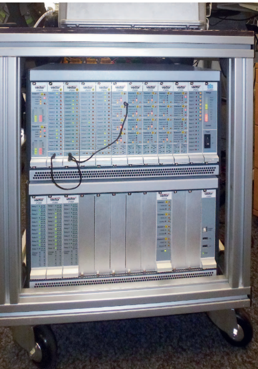
FIGURE 2 Test setup at Claas for measuring and stimulating voltages at ECU pins with the VT System from Vector (© Claas)
